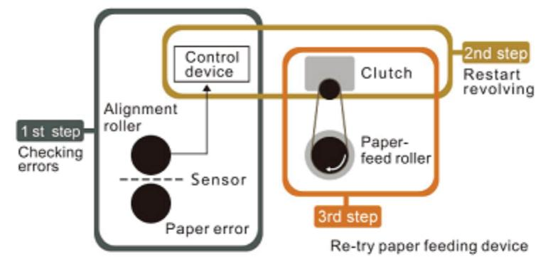
Innovative double-roller paper feed design provides much greater stability, ensuring smooth, reliable feeding. The rollers engage simultaneously so each sheet is fed accurately — one page at a time, every time.
